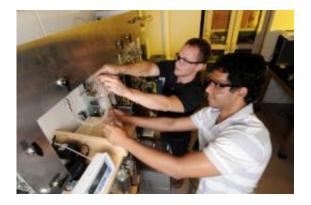
Miles Sakwa-Novak and Ambarish Kulkarni, both Georgia Tech Ph.D. candidates, set up a steam stripping system that can measure the carbon dioxide adsorption and desorption properties of powder samples. Steam stripping is used in adsorbent regeneration. Credit: Georgia Tech Photo: Gary Meek
