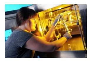
Stephanie Didas, a Georgia Tech Ph.D. candidate, loads an aminosilica sample into a custom-built volumetric adsorption system for measuring adsorption isotherms of different carbon dioxide capture materials. Credit: Georgia Tech Photo: Gary Meek
