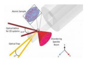
Two thin planes of cold atoms are held in an optical lattice by an array of laser beams. Still another laser beam, passed through a diffusing material, adds an element of disorder to the atoms in the form of a speckle pattern. Credit:
