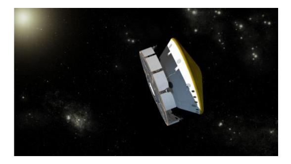
This is an artist's concept of NASA's Mars Science Laboratory spacecraft during its cruise phase between launch and final approach to Mars. The spacecraft includes a disc-shaped cruise stage (on the left) attached to the aeroshell. The spacecraft's rover (Curiosity) and descent stage are tucked inside the aeroshell. Credit: NASA/JPL-Caltech
