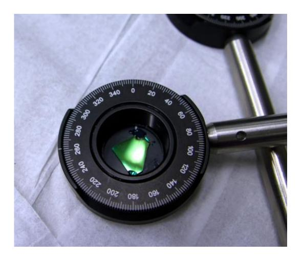
This thin green crystal, developed by a company in Switzerland, is used to convert near-infrared laser light into terahertz frequencies, which are useful for a range of experiments. (Photo by Glenn Roberts Jr.)
