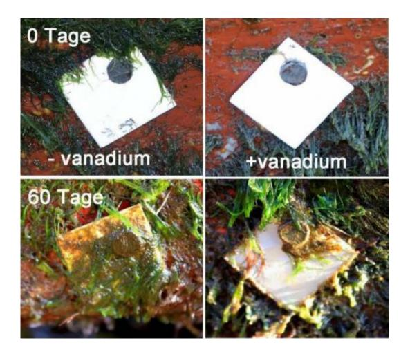
Commercially available antifouling paint with and without vanadium pentoxide nanoparticles was applied to two stainless steel plates (2 x 2 cm). Both plates were attached to a boat moored in a lagoon with direct exposure to Atlantic seawater. After 60 days, the plate without vanadium pentoxide nanoparticles (left) showed heavy fouling; in contrast, the plate with the vanadium pentoxide coating did not (right). Credit: Tremel research group, JGU
