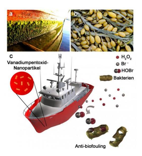
Biofouling at a boat hull; b knotted wrack, Ascophyllum nodosum; c Mode of action of bioinspired under water paints: Like the natural enzyme vanadium
