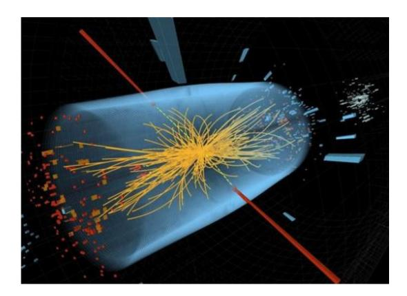
This undated image made available by CERN shows a typical candidate event including two high-energy photons whose energy (depicted by red towers) is measured in the CMS electromagnetic calorimeter. The yellow lines are the measured tracks of other particles produced in the collision. The pale blue volume shows the CMS crystal calorimeter barrel. (AP Photo/CERN)
