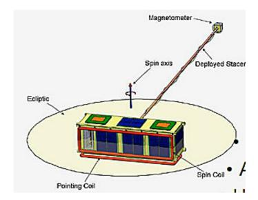
A diagram of the three-cube nanosatellite CINEMA, with its magnetometer boom deployed.
