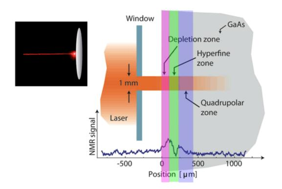
In this illustration, a laser beam is fired through a one millimeter slit at the surface of a gallium arsenide semiconductor. The circularly-polarized light affects the nuclear spin states of the material to a depth of almost 500 microns, about one-half a millimeter.
