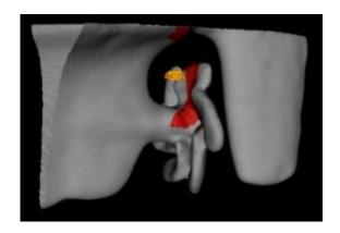
Algorithms developed by MIT researchers enable an autonomous underwater vehicle (AUV) to swim around and reconstruct a ship's propeller. Image: Franz Hover, Brendan Englot
