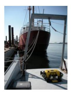
The MIT AUV (in yellow) is designed to swim around the complex structures on a ship's hull to detect small mines. The AUV navigated around the Nantucket Lightship in Boston Harbor during a test run in June 2011. Photo: Brendan Englot
