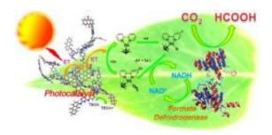
Illustration of the artificial photosynthesis system using a graphene-based photocatalyst to produce formic acid from carbon dioxide under visible light. Image credit: Yadav, et al. ©2012 American Chemical Society
