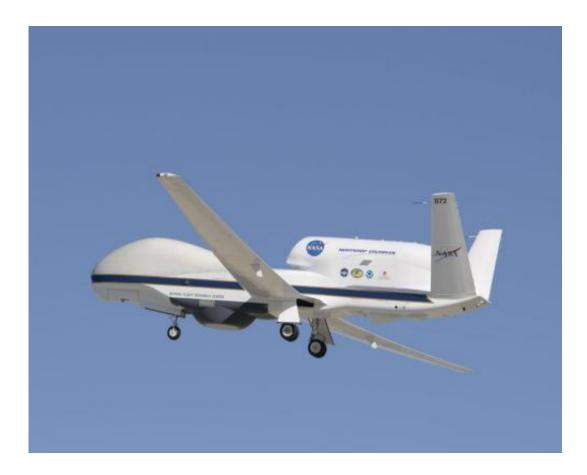
NASA's Global Hawk soars aloft from Edwards Air Force Base, Calif. The NASA Global Hawk is well-suited for hurricane investigations because it can over-fly hurricanes at altitudes greater than 60,000 feet with flight durations of up to 28 hours - something piloted aircraft would find nearly impossible to do. Credit: ED-10-0233-22 Credit: NASA/Tony Landis
