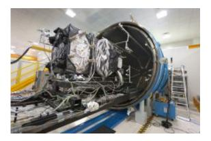
The fourth Galileo In-Orbit Validation flight model satellite, FM4, pictured at the start of thermal vacuum testing at Thales Alenia Space Italy's facility in Rome in May 2012. The third Galileo flight model, FM3, had already undergone this testing. Credits: ESA/EADS Astrium - R. Kieffer
