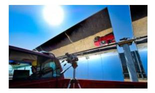
At SkyFuel Inc.'s testing facility in Arvada, Colorado, NREL Engineer Allison Gray drives a pickup truck equipped with Thermal Scout, a device that teams a GPS unit on the roof with an infrared camera in the pickup bed. NREL colleague Benjamin Ihas checks the readings on a laptop to the right of the driver's seat. Credit: Dennis Schroeder
