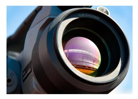
The infrared camera used in Thermal Scout can identify and analyze bad receiver tubes at the speed at which a truck can rumble down the rows of mirrors at a CSP plant. Credit: Dennis Schroeder
