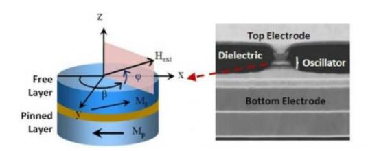
Schematic representation of a spin-transfer nano-oscillator (STNO) with free and pinned magnetic layers (left), and a scanning-electron-microscopy (SEM) image of a cross-section of an STNO (right), showing top and bottom metallic electrodes used for electrical connections. The lateral size of the STNO is about 100nm. (Image courtesy of UCLA Engineering)
