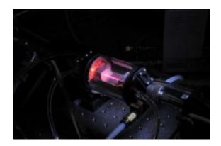
This image depicts the experimental setup used to create a coherent version of the Roentgen tube in the soft X-ray region of the spectrum. When a longwavelength, femtosecond laser is focused into this hollow waveguide filled with high-pressure helium gas, part of the laser is converted into an ultrafast, laserlike, X-ray beam. Credit: Tenio Popmintchev, JILA and University of Colorado at Boulder
