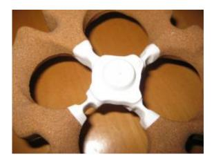
SwRI's Hybrid Ceramic-Sand Core Casting Technology, developed with Grainger and Worrall, Ltd. of the United Kingdom, combines aerospace ceramic and automotive sand core casting processes for precision casting of automotive cast iron/steel components. The technology won a 2012 R&D 100 Award. Credit: Courtesy of Southwest Research
