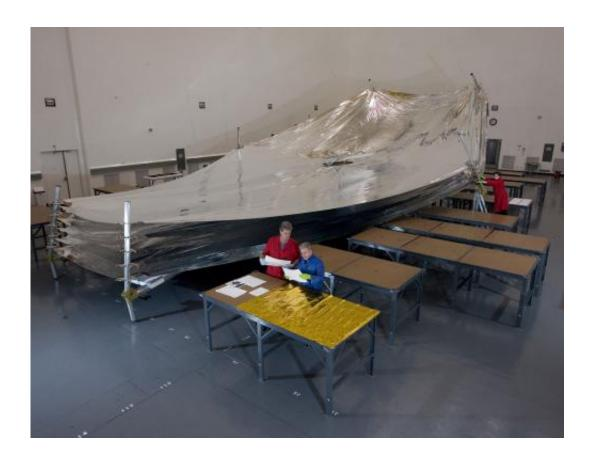
The five-layer James Webb Space Telescope sunshield consists of thin membranes made from a polymer-based film and supporting equipment such as spreader bars, booms, cabling, and containment shells. Designed to block solar light and keep the Observatory operating at cryogenic temperatures. Credit: NASA/Northrop Grumman
