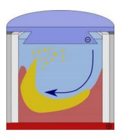
The Tayler instability also affects large-scale liquid metal batteries, which, in the future, could be used for renewable energy storage. Credit: HZDR
