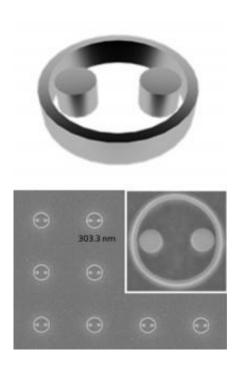
Scheme (top) of the dual-disk ring structure and scanning electron micrscosopy images of fabricated devices (bottom). Credit: Reproduced with permission, 2011 Optical Society of America
