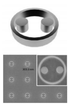
Scheme (top) of the dual-disk ring structure and scanning electron micrscosopy images of fabricated devices (bottom). Credit: Reproduced with permission, 2011 Optical Society of America
