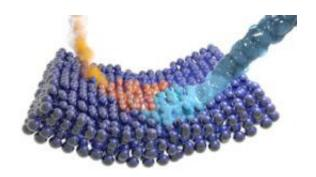
Schematic representation of a membrane failure (red impact) immediately repaired by water flowing through it (blue). © Damien Quémener
