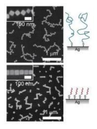
UC San Diego Nanoengineers have developed a technique that enables silver nanocubes to self-assemble into larger-scale structures for use in antennas and lenses. Credit: Tao Research Group, UC San Diego Jacobs School of Engineering.
