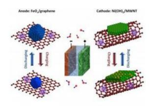
Stanford scientists have developed an ultrafast Edison battery by growing iron oxide crystals on graphene sheets and nickel hydroxide crystals on multi-walled carbon nanotubes. Credit: Hialiang Wang, Stanford University
