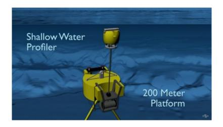
The shallow profiler will float to the surface and get pulled back down to the floating platform by a winch. Credit: CEV/U. of Washington
