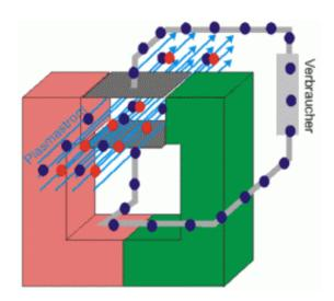
Pictured here, MHD generates electricity directly from a body of very hot moving ionized gas without any mechanical moving parts. Solar energy, concentrated by mirrors and lenses, creates superheated gases; magnetohydrodynamics works by using superconducting magnets to extract electricity from the superheated moving ionized gas.
