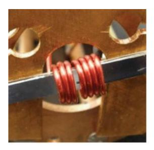
Close up of the mount used to hold a gallium arsenide (semiconductor) sample, showing the radio-frequency coil used for pulsed spin manipulation. (Credit: Yunpu Li)
