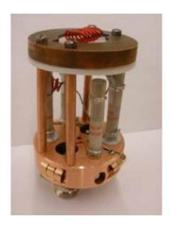
The probe head used to send radio-frequency pulses onto the coil used for pulsed spin manipulation of a gallium arsenide (semiconductor) sample. (Credit: Yunpu Li)
