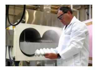
Kevin Keener developed a rapid egg cooling system that uses circulated carbon dioxide to create a thin layer of ice inside an egg's shell that cools the inside of an egg within minutes, strengthening proteins and increasing shelf life. Credit: Purdue Agricultural Communication file photo/Keith Robinson
