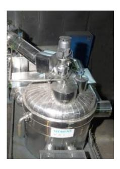
Heat recovery plant installed by Siemens in the electric steel plant of Stahlwerk Thüringen GmbH in Unterwellenborn (Germany). The pilot plant runs with molten salt, and is used for material validation and process optimization.
