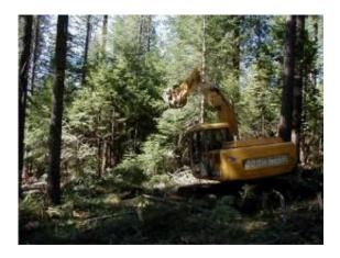
A masticator is used to mechanically thin a mixed-conifer forest in the central
