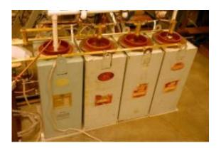
Four capacitors supply up to 10,000 volts of energy to separate the xenon electrons from their nuclei, creating an electrically charged plasma. Credit: U. of Washington
