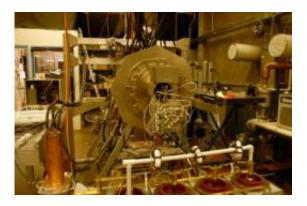
The lab equipment includes a small system that measures plasma for electronics applications, attached to a larger tank containing plasma for energy research. Credit: U. of Washington
