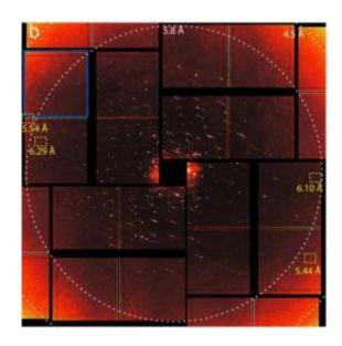
X-ray diffraction patterns of photosystem II microcrystals obtained at the Linac Coherent Light Source were reconstructed by computers into images of the composition and atomic structure of the crystals at a resolution of 6.5 angstroms, the first ever such images at room temperature. Credit: Images courtesy of SLAC
