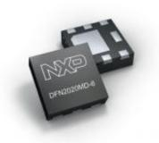
NXP Semiconductors today introduced the industry's first MOSFETs in a 2-mm x 2-mm low-profile DFN (discrete flat no-leads) package with tin-plated, solderable side pads. These unique side pads offer the advantage of optical soldering inspection, as well as a better quality of solder connection compared to conventional leadless packages.
