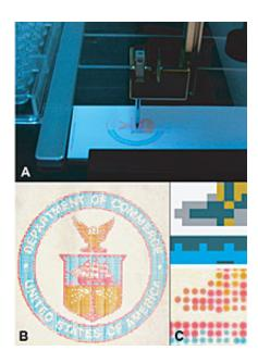
Microarrayer machines (A) now can mix colors and deposit them on microscope slides, which can be used to calibrate hyperspectral imagers (HSI) for use in medical applications. The finished slides can be custom-colored (B) to calibrate HSIs to find specific types of tumors or disease tissue. Close up, they resemble dot-matrix printwork (C). Credit: Clarke/NIST
