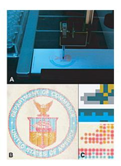
Microarrayer machines (A) now can mix colors and deposit them on microscope slides, which can be used to calibrate hyperspectral imagers (HSI) for use in medical applications. The finished slides can be custom-colored (B) to calibrate HSIs to find specific types of tumors or disease tissue. Close up, they resemble dot-matrix printwork (C). Credit: Clarke/NIST
