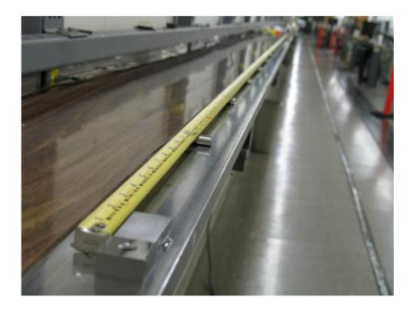
Researchers calibrate measuring tapes of all types in the 60-meter long NIST tape tunnel. Credit: NIST
