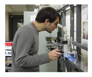
NIST technician Christopher Blackburn uses a microscope to precisely align a retroreflector over the center of a hash mark on a measuring tape. Photo credit: Bruce Borchardt
