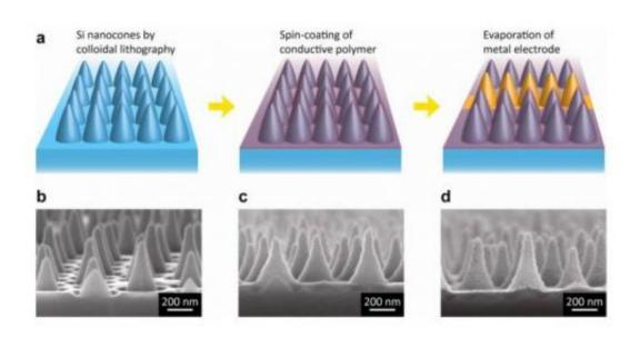
(a) Fabrication process of the solar cells, in which silicon nanocones are coated with a polymer. (b), (c), and (d) show scanning electron microscope images of the nanocones after each step. Image credit: Jeong, et al. ©2012 American Chemical Society
