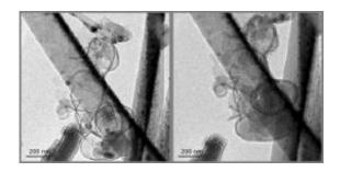
In situ transmission electron microscopy at EMSL was used to study structural changes in the team's new anode system. Real-time measurements show silicon nanoparticles inside carbon shells before (left) and after (right) lithiation.
