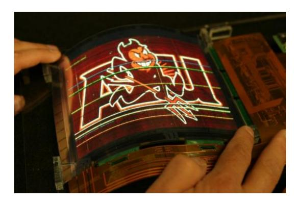
Researchers at the Flexible Display Center at ASU have successfully manufactured the world's largest flexible color organic light emitting display prototype using advanced mixed oxide thin film transistors. Photo by: Jann Kaminski, ASU
