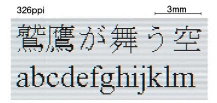
(Phys.org) -- Japan Display Inc. has created a small direct-view display that is packed with so many pixels that it features twice the resolution of
