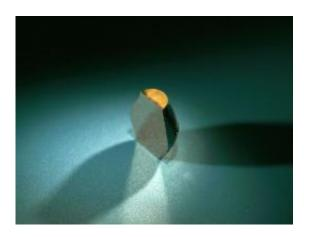
An alternative to precious metal: Max Planck scientists used this crystal of an iron-aluminium compound to catalyse an important step in the production of polyethylene plastic. To date, industry has used a palladium compound for this process. © MPI for Chemical Physics of Solids
