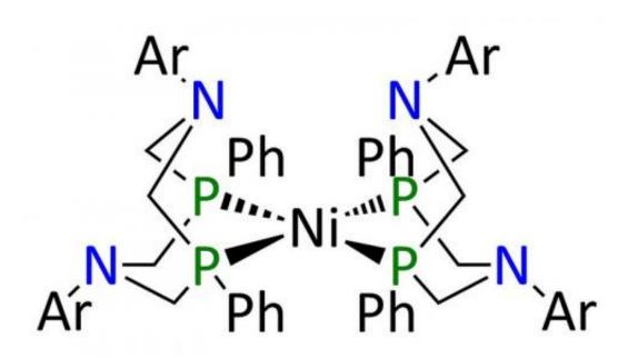
Combined with an acidic ionic liquid, this catalyst can make hydrogen gas fast and efficiently.
