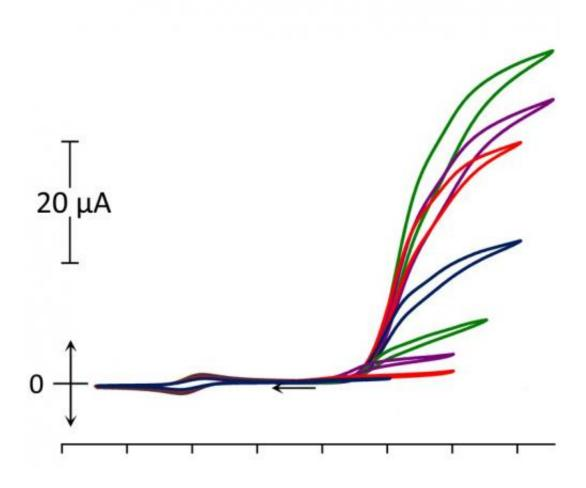
This graphic roostertail illustrates how the catalyst picks up speed as water is added to the ionic liquid (more water equals taller, faster current)
