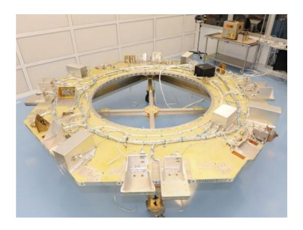
An instrument deck for NASA's Magnetospheric Multiscale mission is readied for installation of instruments. Two instruments have already been installed: the white box on the lower right is the Energetic Ion Spectrometer; the black box in the upper right is the Central Instrument Data Processor. Credit: NASA\GSFC\Lambert
