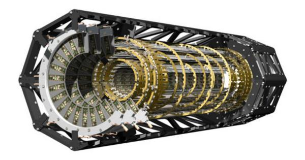
ATLAS's innermost detector consists of three barrels, the diameter of the outermost equalling 24 centimeters (less than 10 inches), plus three disks; 80 million pixels cover an area of 1.7 square meters (18 square feet). Particle tracks are followed through three layers of pixels, initiating precise measurement of each event.
