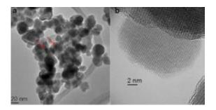
Figure: Representative transmission electron microscope (TEM) images of graphene nanoparticles (a-b). The dark spots (red arrow) in panel (a) are the manganese ions intercalated between the graphene sheets. The high resolution TEM images (b) show the planar graphene lattice planes.
