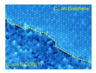
STM three-dimensional rendered image of a C60 self-assembled monolayer at a domain boundary of graphene and bare SiC(0001); each C60 molecule is 1 nm in diameter.
