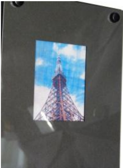
A color image displayed on the prototyped e-paper
