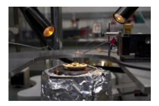
Shriram Ramanathan's laboratory setup for testing solid-oxide fuel cells. The fuel cell is hidden under the circular component at the top, which pins it down to create a tight seal with the hydrogen fuel entering from below. Two needles connect with the electrodes to measure the electricity produced. Credit: Caroline Perry, Harvard SEAS
