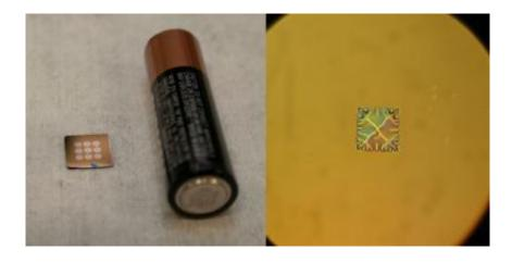
Left: Each dark speck within the nine white circles at left is a tiny fuel cell. An AA battery is shown for size comparison. Right: One of the nine circles is magnified in this image, showing the wrinkled surface of the electrochemical membrane. Credit: Left: Caroline Perry, SEAS Communications. Right: Quentin Van Overmeere, Harvard SEAS.
