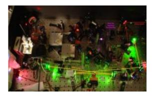
This colorful apparatus is a key part of the JILA frequency comb instrument used to measure trace gases for biomedical applications. The beam from a powerful fiber laser is converted by a special crystal and other optics into two light waves at lower frequencies. The system can detect and measure the concentration of many different molecules based on how they absorb light in the mid-infrared region of the electromagnetic spectrum. Credit: JILA
