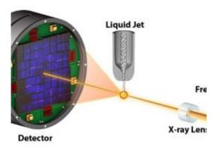
Schematic representation of the experimental setup at the Coherent X-ray Imaging endstation at the Linac Coherent Light Source. Millions of tiny crystals are injected into the free-electron laser beam in a thin liquid jet. Diffraction patterns are generated when a crystal intersects a free-electron X-ray flash and are captured on a detector shown on the left.
