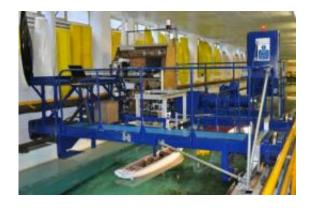
This image shows tow tank testing of the B9 fossil fuel free ship. Credit: University of Southampton
