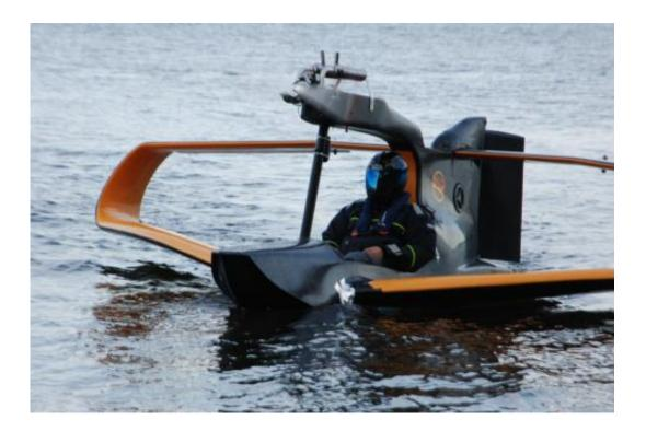
(Phys.org) -- A single-seat carbon-fiber airplane designed for water operations and proposed as a "fun flyer" has taken its first test flight at Finland's Lake Hepari. The June test flight comes after more than a year since its introduction at an air show in Germany in 2011. The <u>earlier</u> <u>FlyNano</u> was showcased as a single-occupant petrol/electric microlight amphibious aircraft. The new FlyNano has undergone key changes to
