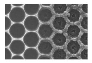
A composite image showing (left) an alumina-based honeycomb lattice with approximately one micron diameter cells, from which (right) an equivalent porous coordination polymer (PCP) architecture is derived using "reverse fossilization." Credit: Kyoto University iCeMS
